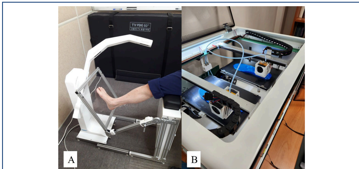
Figure 1. Equipment to create customized 3D-printed insole orthoses: (A) MediAce scan 3D scanner instrument; (B) 3D printer instrument to produce final insole orthoses for LLD correction.
